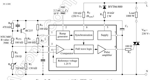
Figure 9. Temperature control 15 to 35°C with sensor monitoring NTC–Sensor M 87 Fabr. Siemens
