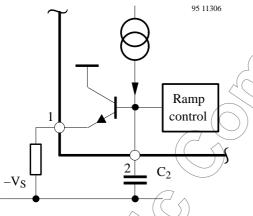
Figure 2. Pin 1 internal network
